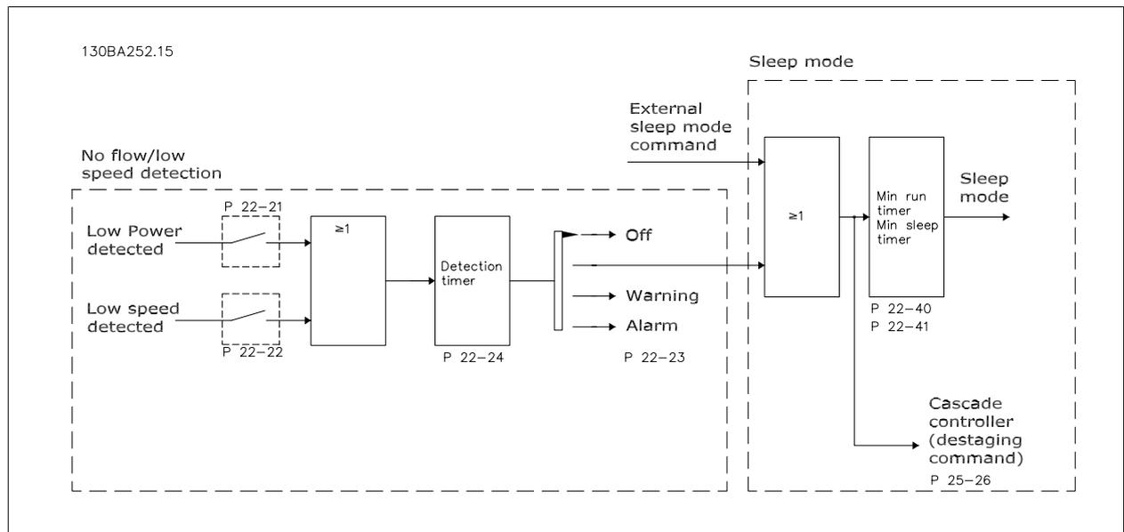
The VLT AQUA Drive includes functions for detecting if the load conditions in the system allow the motor to be stopped:
