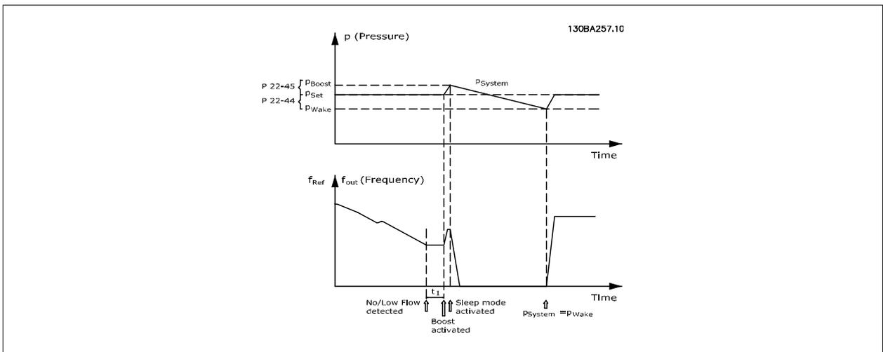
If no flow is detected, the frequency converter will increase the set point for pressure to ensure a slight over pressure in the system (boost to be set in par. 22-45, *Setpoint Boost*).
