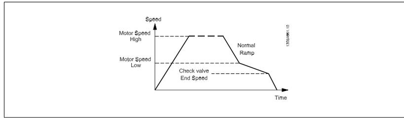
**3-87 Check Valve Ramp End Speed [Hz]**
