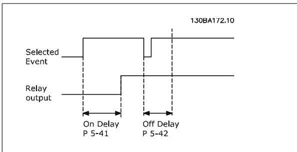
If the selected Event condition changes before the on- or off delay timer expires, the relay output is unaffected.
