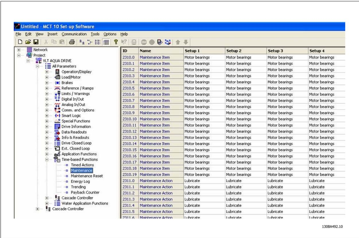
The LCP indicates (with a wrench-icon and an "M") when it is time for a Preventive Maintenance Action, and can be programmed to be indicated on a digital output in parameter group 5-3\*. The Preventive Maintenance Status may be read in par.16-96 *Maintenance Word*. A Preventive Maintenance indication can be reset from a digital input, the FC bus or manually from the LCP through par.23-15 *Reset Maintenance Word*.
