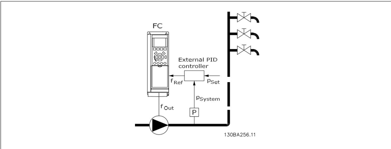
2) In systems where the pressure or temperature is controlled by an external PI controller, the wake up conditions can not be based on feedback from the pressure/temperature transducer as the setpoint is not known. In the example with a boost system, desired pressure  $P_{Set}$  is not known. Par. 1-00, *Configuration mode*, must be set for Open Loop.
