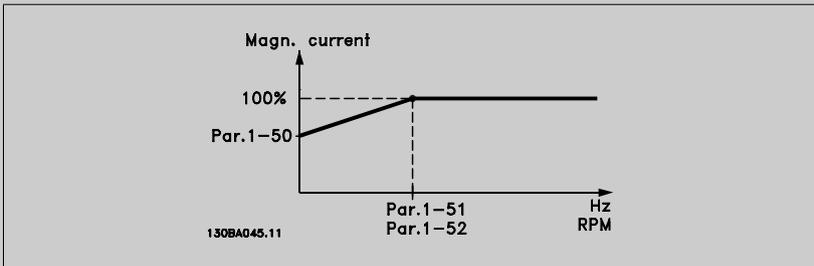
**1-51 Min Speed Normal Magnetising [RPM]**
