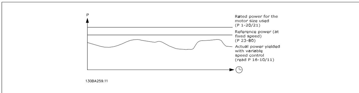
The difference between the Reference Power at fixed speed and the Actual Power yielded with speed control represent the actual saving.
