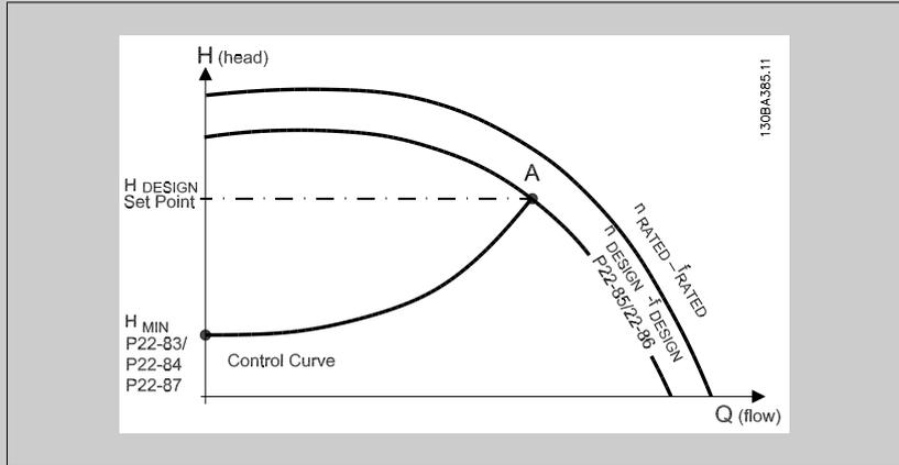
From the data sheet showing characteristics for the specific equipment at different speeds, simply reading across from the  $H_{DESIGN}$  point and the  $Q_{DESIGN}$  point allows us to find point A, which is the System Design Working Point. The pump characteristics at this point should be identified and the associated speed programmed. Closing the valves and adjusting the speed until  $H_{MIN}$  has been achieved allows the speed at the no flow point to be identified.
