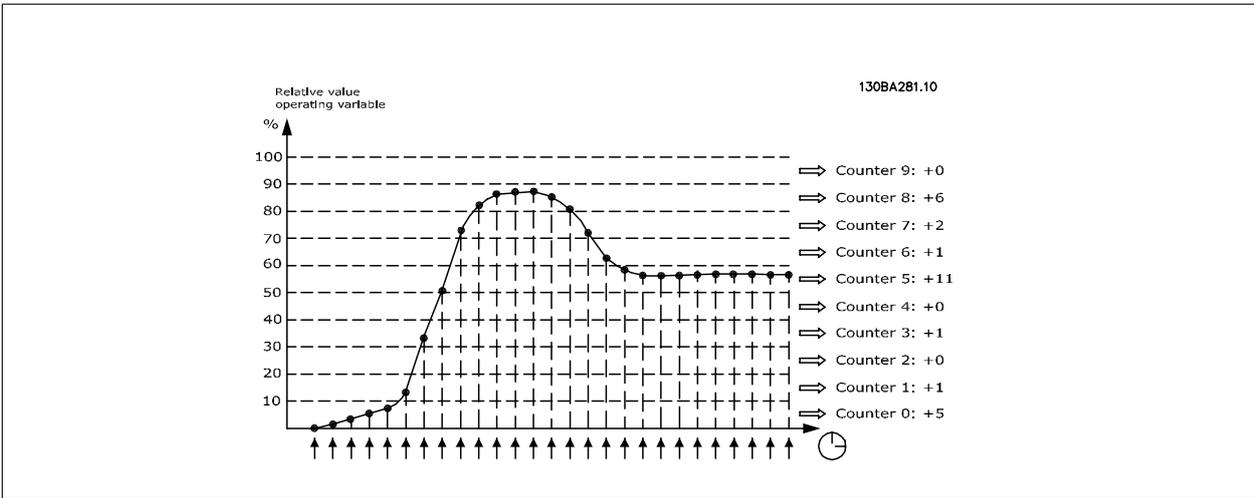
Once a second, the value of the operating variable selected is registered. If a value has been registered to equal 13%, the counter "10% - <20%" will be updated with the value "1". If the value stays at 13% for 10s, then "10" will be added to the counter value.
