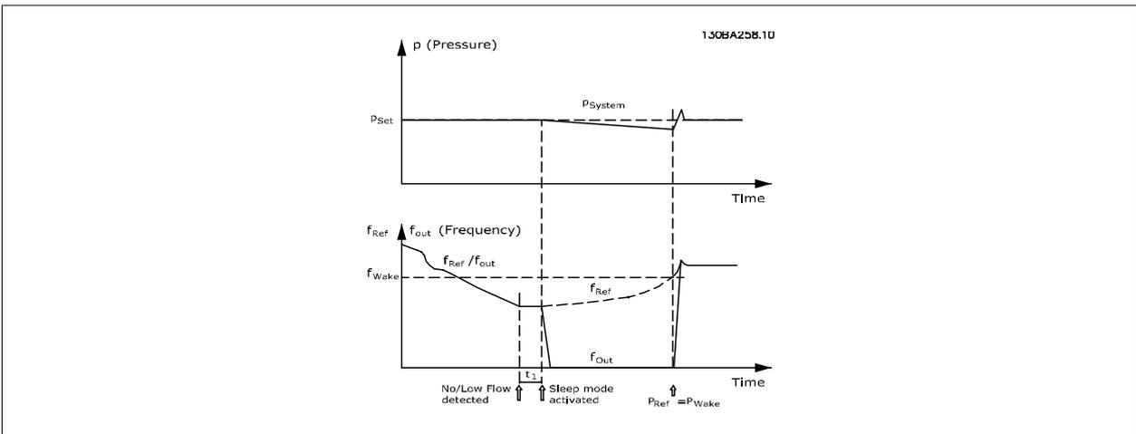
When low power or low speed is detected the motor is stopped, but the reference signal ( $f_{ref}$ ) from the external controller is still monitored and because of the low pressure created, the controller will increase the reference signal to gain pressure. When the reference signal has reached a set value  $f_{wake}$  the motor restarts.
