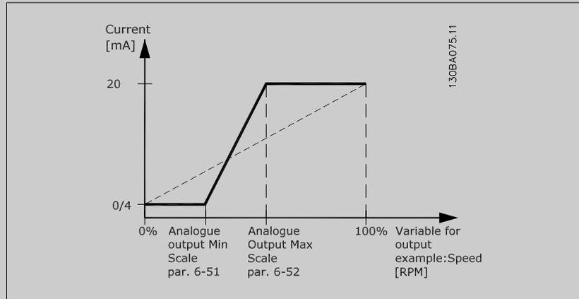
It is possible to get a value lower than 20 mA at full scale by programming values >100% by using a formula as follows:
