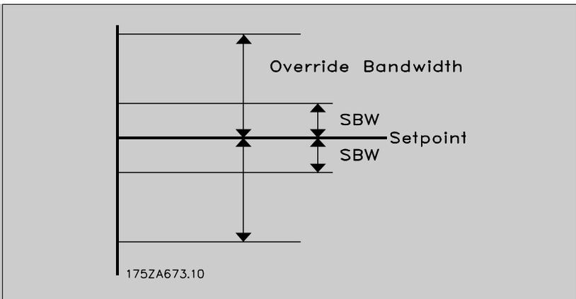
Setting the OBW too close to the SBW could defeat the purpose with frequent staging at momentary pressure changes. Setting the OBW too high might lead to unacceptably high or low pressure in the system while the SBW timers are running. The value can be optimized with increased familiarity with the system. See par.25-25 *OBW Time*.
