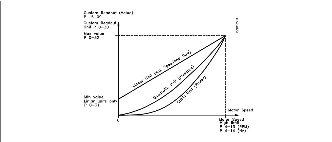
The relation will depend on the type of unit selected in par.0-30 *Custom Readout Unit*.
