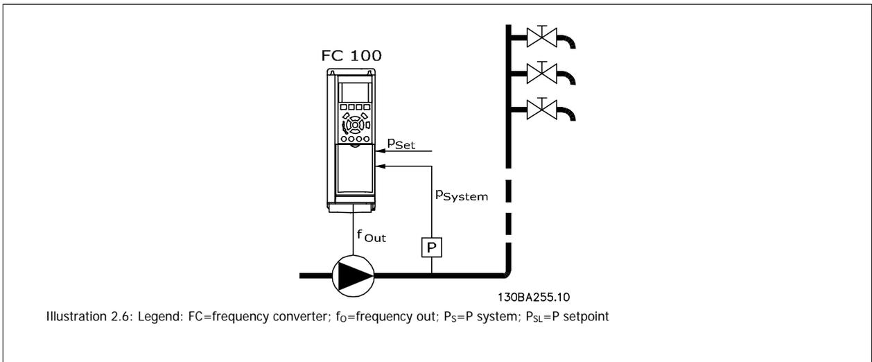
1) Systems where the integrated PI controller is used for controlling pressure or temperature e.g. boost systems with a pressure feed back signal applied to the frequency converter from a pressure transducer. Par. 1-00, *Configuration Mode*, must be set for Closed Loop and the PI Controller configured for desired reference and feed back signals.
