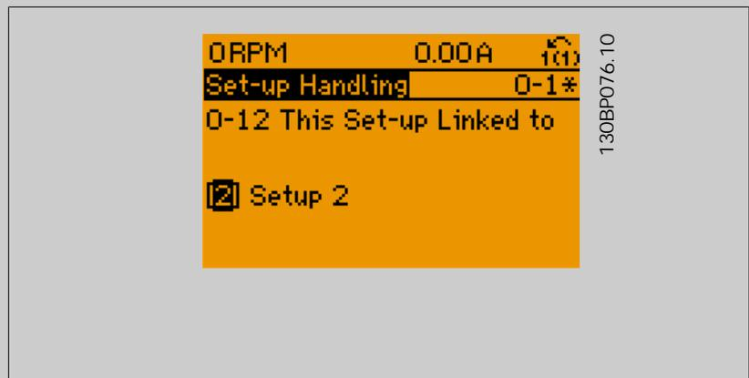
After the link is complete, par.0-13 *Readout: Linked Set-ups* will read {1,2} to indicate that all 'not changeable during operation' parameters are now the same in Set-up 1 and Set-up 2. If there are changes to a 'not changeable during operation' parameter, e.g. par.1-30 *Stator Resistance (Rs)*, in Set-up 2, they will also be changed automatically in Set-up 1. A switch between Set-up 1 and Set-up 2 during operation is now possible.
