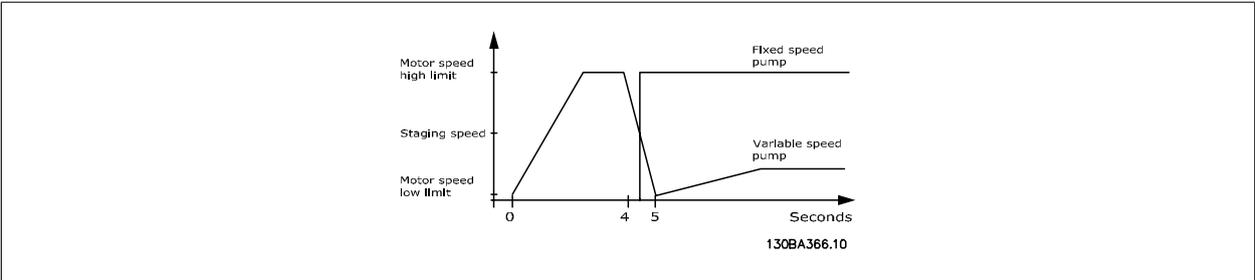
**NB!** If the set-point is reached after staging before the variable speed pump reaches its minimum speed - the system will enter the state closed loop as soon as the feedback pressure is crossing the set-point.
