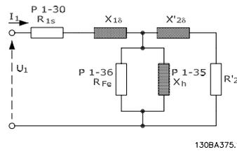
Illustration 2.1: Motor equivalent diagram for an asynchronous motor
