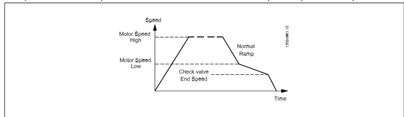
**3-86 Check Valve Ramp End Speed [RPM]**
